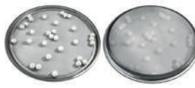
Elastomeric balls anti-blinding device
